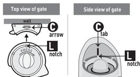
**5c** Align the lower part of gate to Lower Bracket (D) and top of gate to Upper Bracket (C). Push down gently to click into place.
