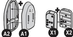
Never use just backing Spacers (A2, X2) to mount gate, they must always be used in conjunction with front Spacers (A1, X1) **!**
