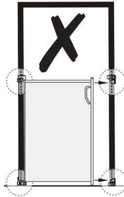
**!** The edge of brackets should **NOT** be over the door frame (or wall) edge after assembling.
