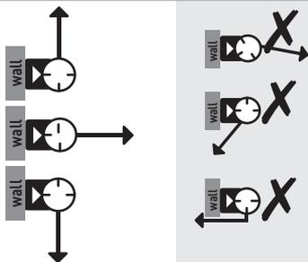
**5b** Align the notch on Top of Casing (L) with the arrow on the Upper Bracket (C) in desired open / close direction.
