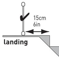
**1d.** If the safety barrier is used at the top of stairs, it should not be positioned below the top level. At the top of landing, position the gate 15cm away from the top step.
