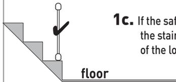
**1c.** If the safety barrier is used at the bottom of the stairs, it should be positioned at the front of the lowest tread possible.
