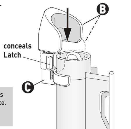
**!** The Cover locks the gate in place. It must be securely installed at all times.
